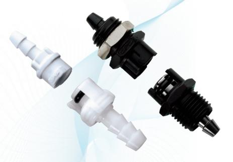
The SMC and SMF1 are among CPC's smallest couplings. These twistto-connect couplings provide a reliable and more secure alternative to luer-type connections. They also allow for the tubing to rotate freely when connected. This important feature prevents both kinked tubing and accidental disconnection during use.
