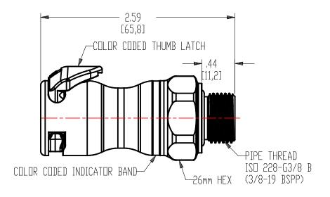
Description: 3/8" G-Thread/BSPP/BSPP Valved In-line Liquid Cooling Body, Warm Red
