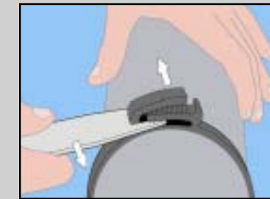
4. To remove the clip, place the HCL removal tool at the bottom part of the female jaw and slide or twist sideways.
